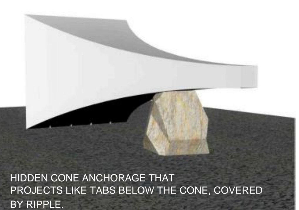
SITUATION OF PLACED ELEMENTS, PRIOR TO APPLICATION OF CRUSHED ROCK (RIPIO): THE LEVEL OF FOUNDATIONS MATCHES THE LEVEL OF LAND WITHOUT AGGREGATE
